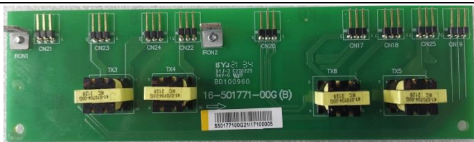
DRV Power board
